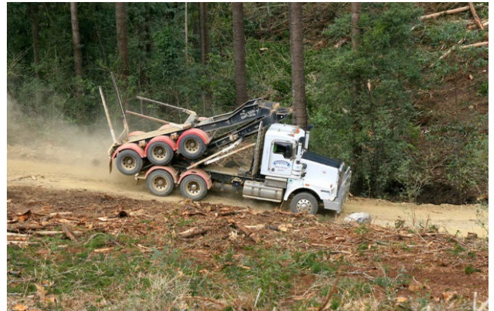
Folding skel truck commonly used for Araucaria logs
