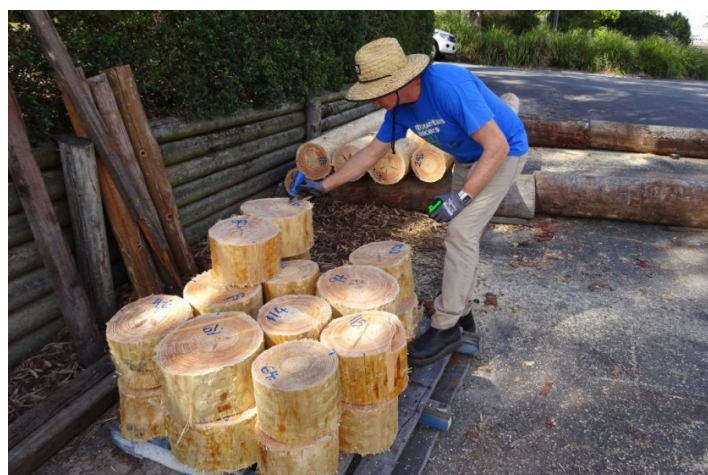
Stem segments being prepared for assessment at DPI's Salisbury facility as part of Southern Pine Resource Characterisation study
