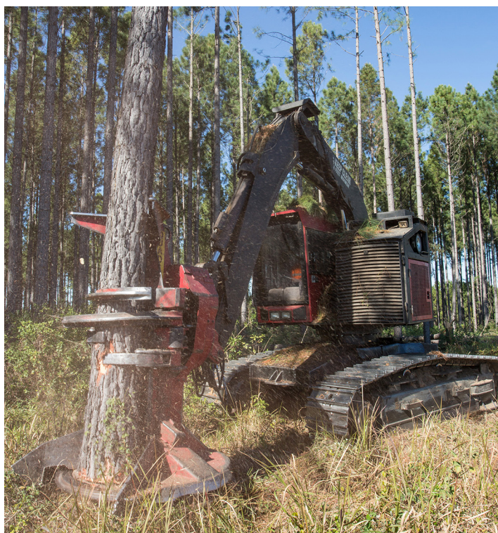
Whole stem harvesting operations can cut and snig 1,500 m 3 per day
