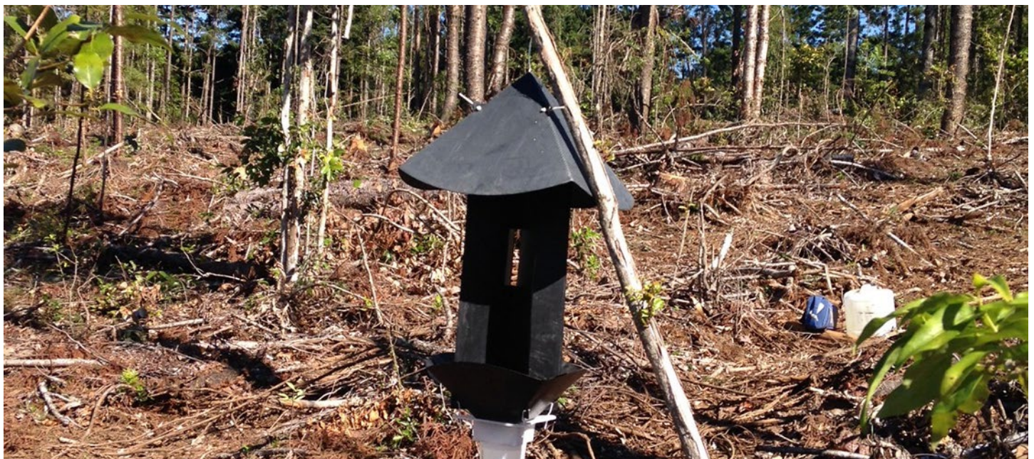
Static panel traps with specific lures are monitored during the flight season to detect the presence of new incursions such as Sirex wood wasp
